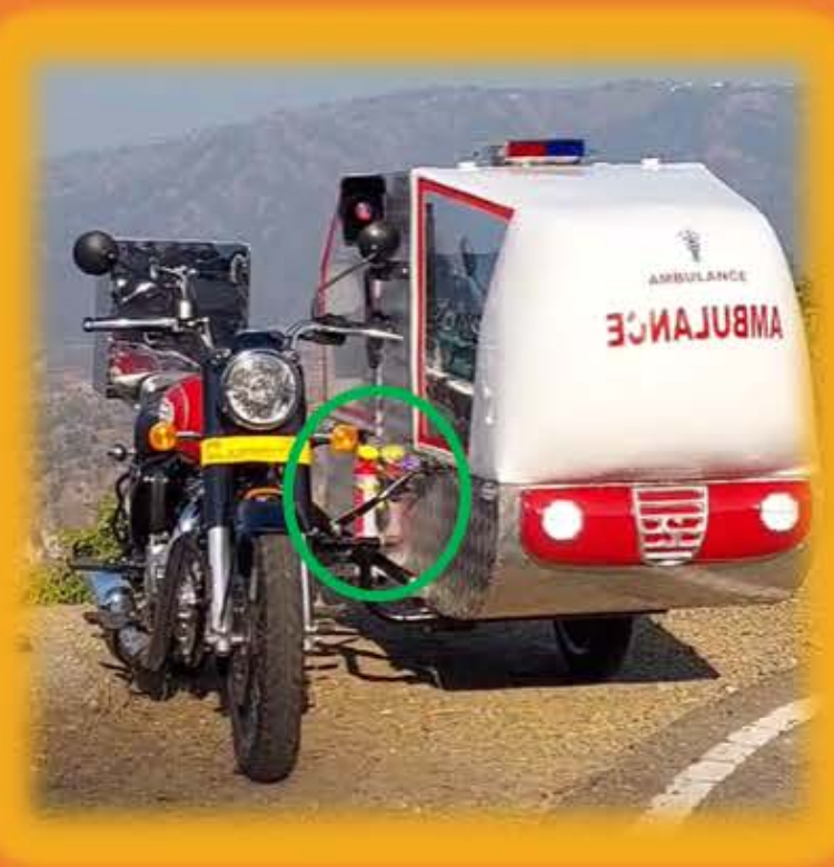
Equipped with Fire Extinguisher to manage fire incidences at Site for rescuing victim
